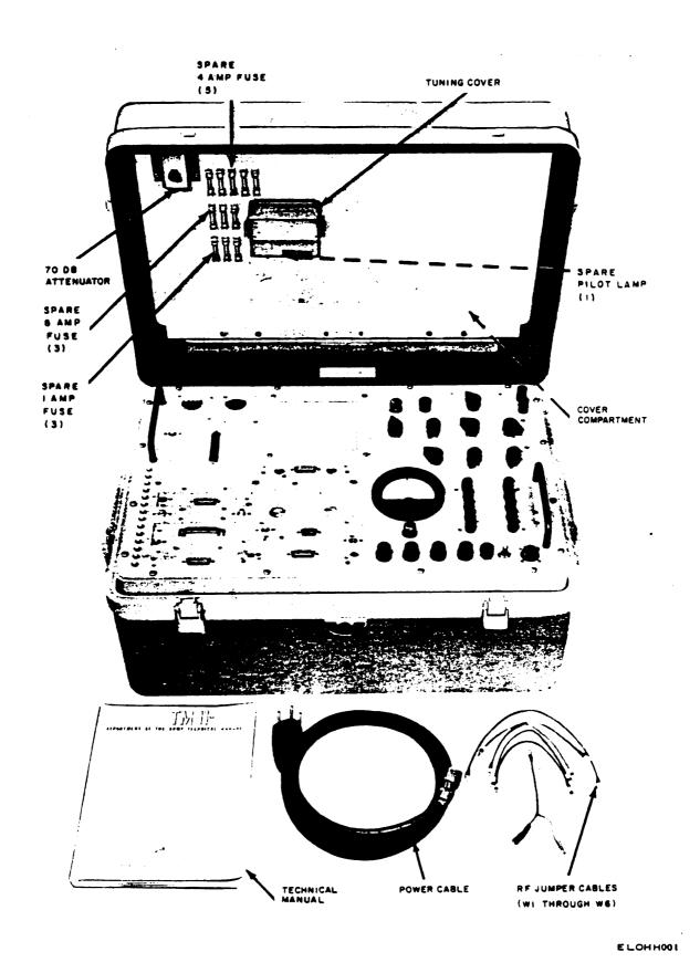
Figure 1-1. Test Set, Electronic Circuit Plug-In Unit AN/ARM-87
