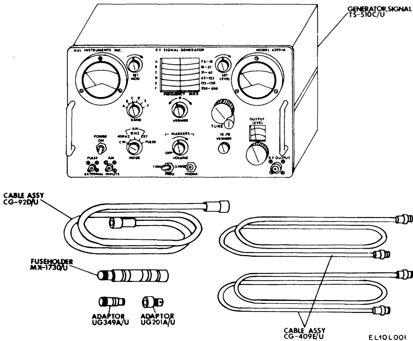
Figure 1-1. Signal Generator AN/USM-44C, less Case CY-7520/USM-44C
