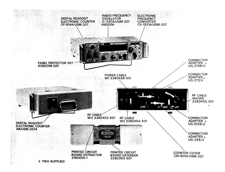
Figure 1-1. Digital Readout Electronic Counter AN/USM-207A
