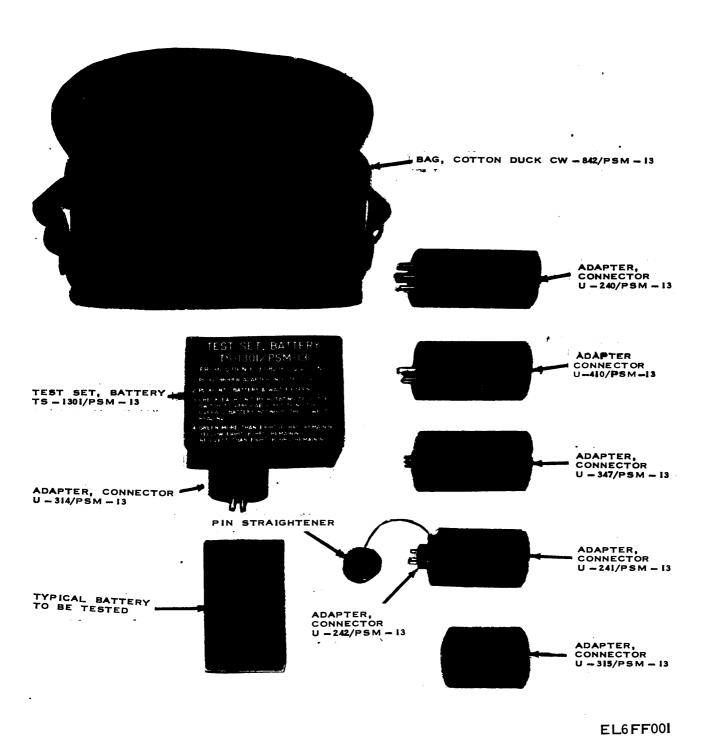
Figure 1-1. Test Set, Battery AN/PSM-13.
