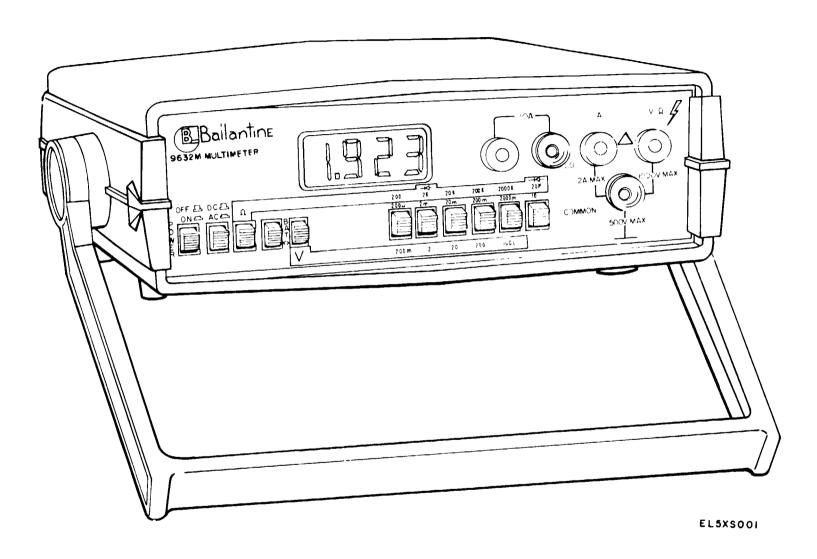
Figure 1-1. Multimeter, AN/USM-451
